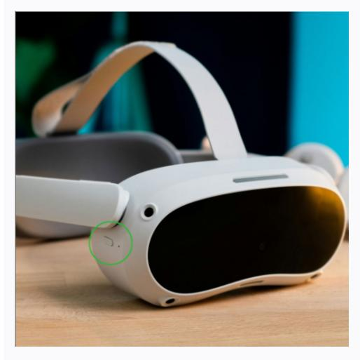
• Power on the headset by pressing the power button for about 2-3 seconds.
